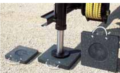
Always use outrigger mats and if in doubt select larger ones to lower ground bearing pressure.
